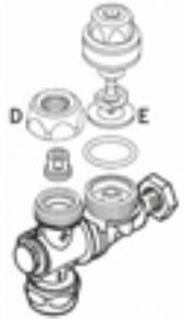
If some nozzle drips when the sectors are being closed, you will have to replace the antidrip diaphragm (E).
