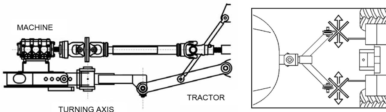
The turning axis will always have to stay much forwards in relationship with the homokinetic knot to avoid that this one makes too closed turns. If needed, an adjustment of the hitching bar will have to be made as it is explained in the chapter of drawbar adjustment.
