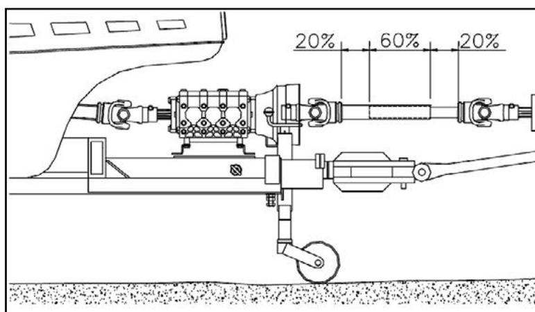
8. Grease the tubes and assemble again the PTO shaft to the tractor and to the machine.
