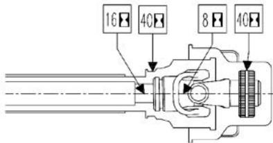
In PTO shafts supplied with homokinetic shafts there are 5 greasing points.
